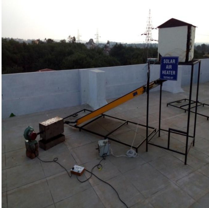
Fig.2 Test set up for solar hybrid maize drying The overall results are represented as under.
