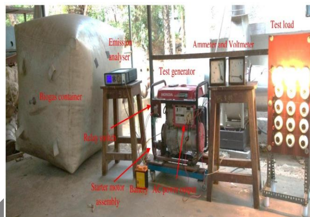
Fig. 2 Experimental set up of LPG generator functioning using biogas
