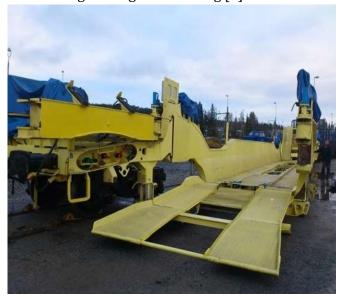
Fig. 1. Specialized wagon in the ready position for loading [4]
