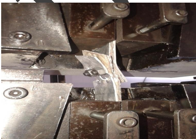
Fig. 9: Actual image of sample breaking condition for tensile testing on UTM machine
