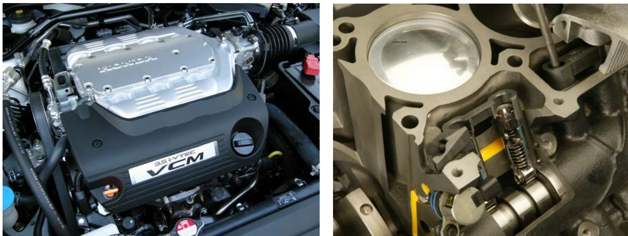
Fig 2. “Variable Cylinder Management” (VCM) system of engine by Honda.
