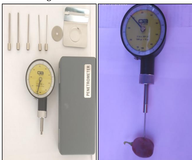
A-grape hardness measuring device B-grape hardness measurement Figure 1. Processes for determining the mechanical composition of grape varieties using instruments
