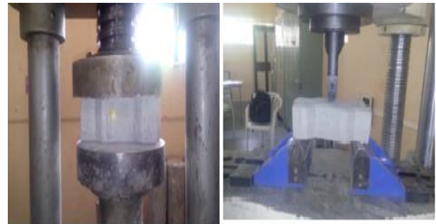
Figure1: Compressive and Flexural Strength Tests
