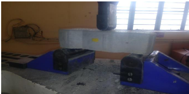
Figure 2: Flexure Test Detail
