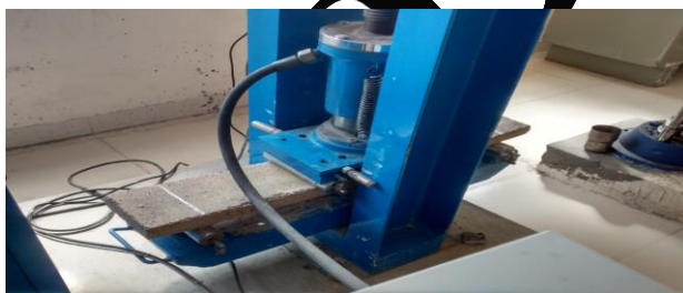
Figure 3-Flexural testing of specimen
