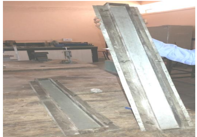
Fig. 1 - Tension Test Mould
