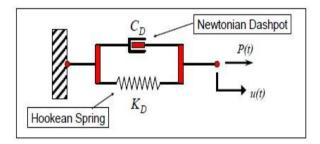
Most of the mathematical properties of VE material is complex and may vary with the environmental temperature and excitation frequency. Hysteresis loop is obtained when VE damper subjected to periodic displacement. Area of hysteresis represents the actual energy loss. The main VD properties used the designing VE damper as storage modulus .G' provide with the actual elastic shear stiffness of material The stress strain relation expressed as
