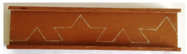
Fig 2.1.1 Marking Pentalpha Perforated beam
