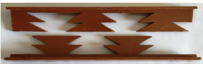
Fig 2.1.5 Cutting Monogram Perforated Beam
