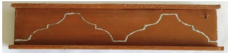
Fig 2.1.7 Marking Pinnacle Perforated Beam
