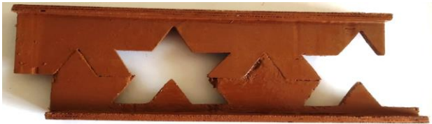
Fig 2.1.3 Final Pentalpha Perforated Beam
