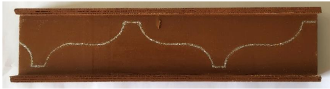
Fig 2.1.10 Marking Pixshark Perforated Beam
