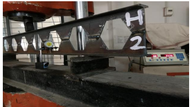
Testing of Hexagonal Prepared Tapered Section (45°)
