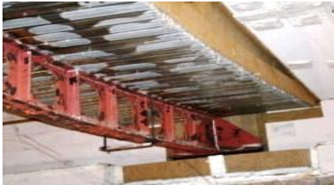
Fig 1. Flexure Buckling of Castellated Beam
