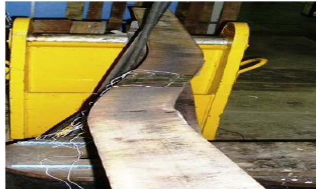
Fig 3 Lateral-Torsional Buckling of Castellated Beam
