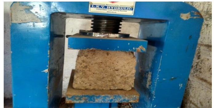
Figure no. 4: Compression testing on specimen
