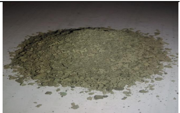
Figure no. 1: Modified Dry mix of e-waste concrete (source-camera)
