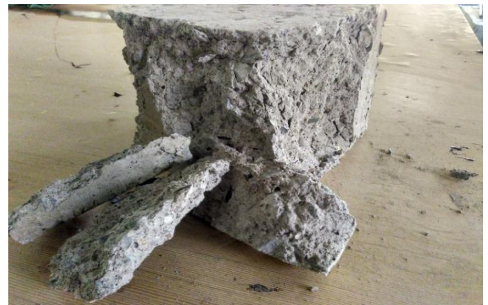
Figure no. 5: Specimen after compression testing
