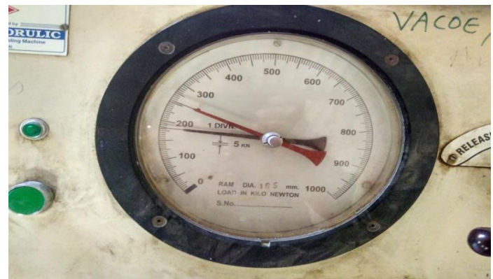
Figure no. 6: Readings on compression testing machine
