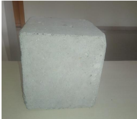
Figure no. 2: concrete cube casted with addition of e-waste and waste foundry sand (source-camera)
