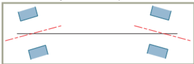
Fig.3.2 Misalignment between centerline of shaft and bearing housing
