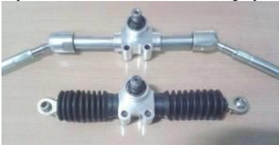
Fig. 2.1 Rack and pinion steering
