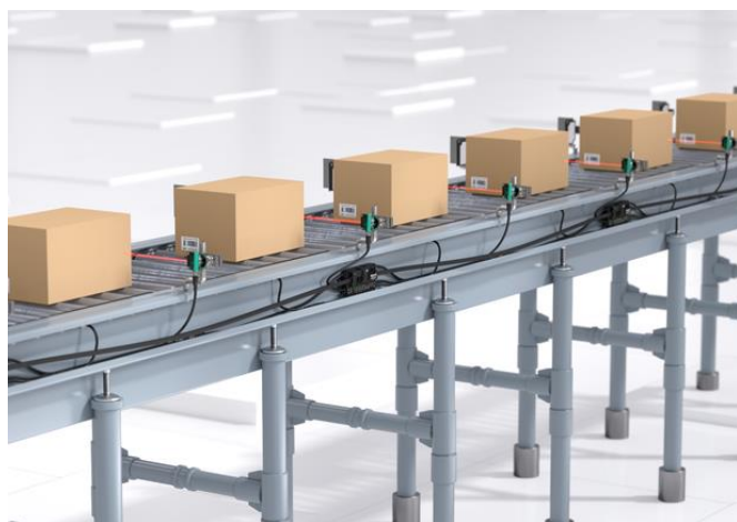
Fig: Automated conveyor system using light emitting sensor
