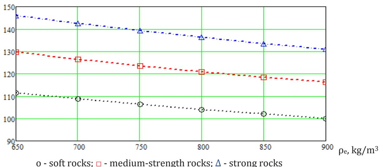
Fig. 1. Change in the diameter of the explosive charge  $d_{ch}$  from the density of the explosives  $\rho_e$  in various rocks
