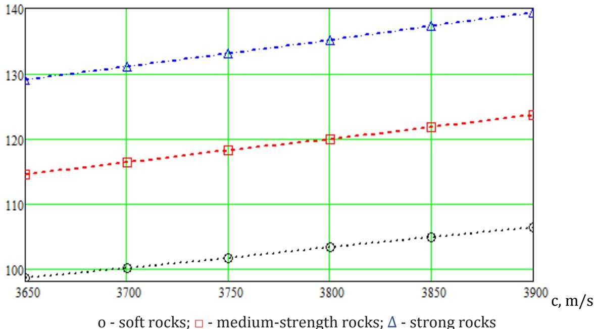
Fig. 3. Change in the diameter of the explosive charge  $d_{ch}$  from the velocity of the longitudinal wave  $C$  in various rocks
