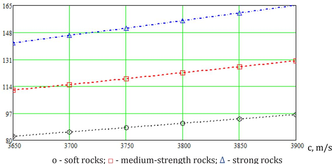
Fig. 5. Change in the linear mass of the charge of a contour well  $\rho$  from the velocity of the longitudinal wave in the rock  $c$  in various rocks
