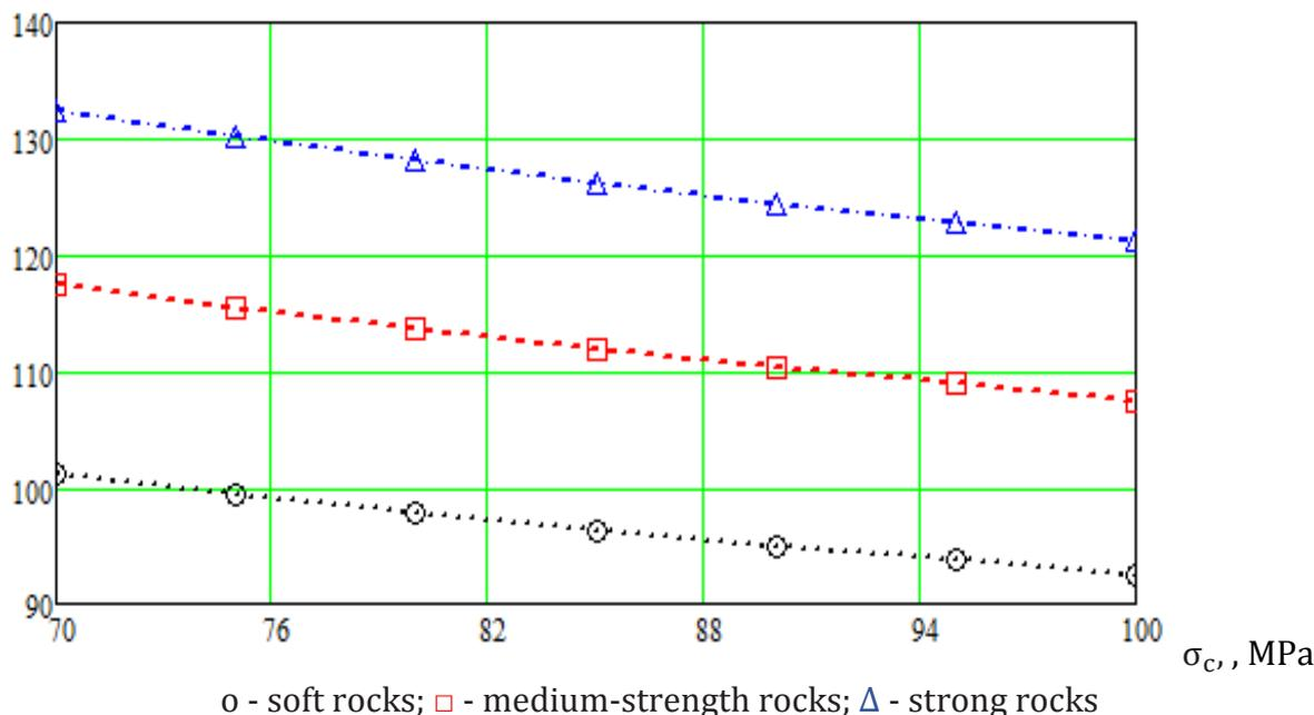
Fig. 2. Change in the diameter of the explosive charge  $d_{ch}$  from the compressive strength of rocks  $\sigma_c$  in various rocks
