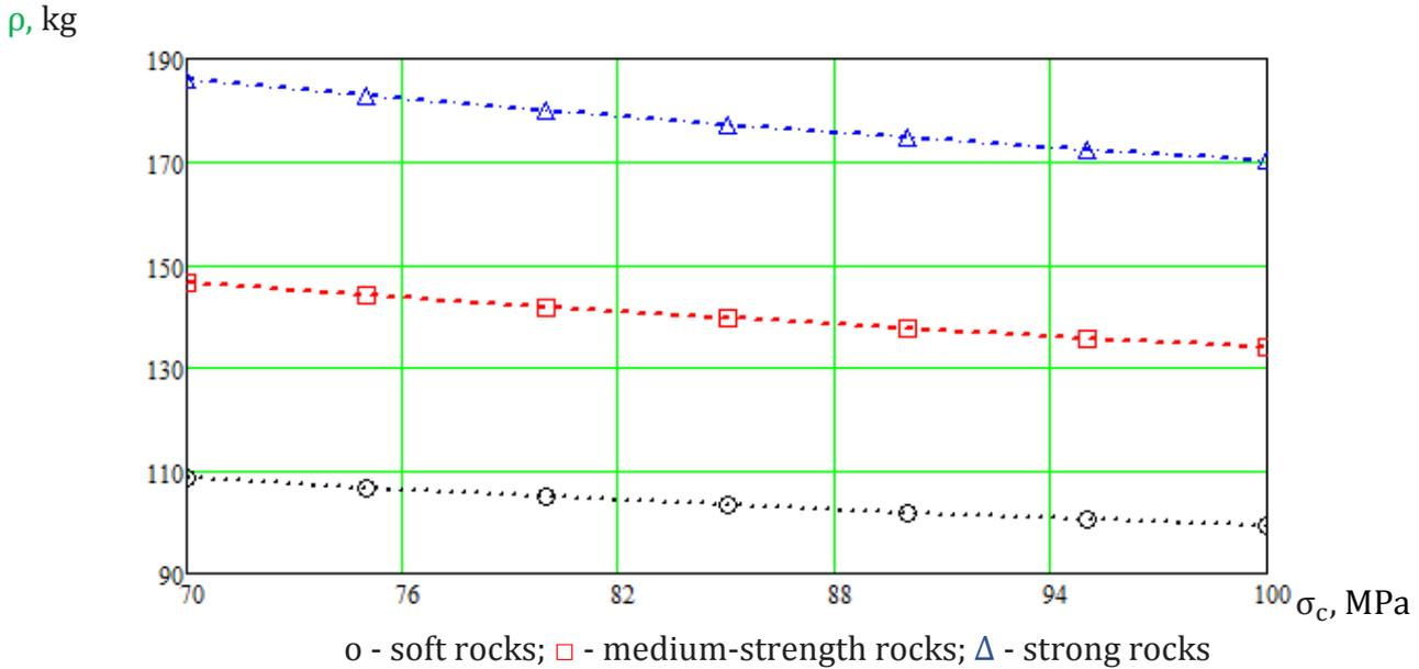
Fig. 8. Change in the linear mass of the contour well charge  $\rho$  from the compressive strength of rocks  $\sigma_c$  in various rocks
