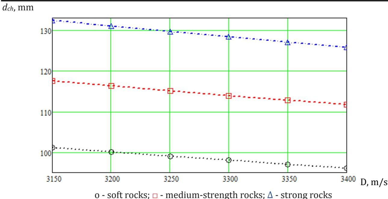
Fig. 4. Change in the diameter of the explosive  $d_{ch}$  charge from the explosive D detonation rate in various rocks
