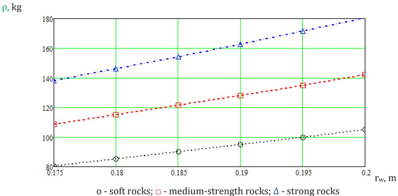
Fig. 9. Change in the linear mass of the contour well charge  $\rho$  from the radius of the contour well  $r_c$  in various rocks
