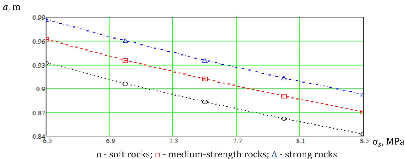
Fig. 13. Variation of the distance between contour wells  $a$  from the tensile strength of rocks  $\sigma_s$  in various rocks
