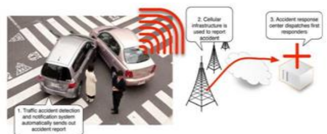
Figure 1. Smartphone Based Accident Detection
