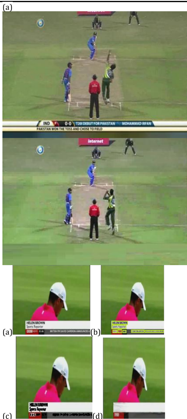
Fig.3. Output results of video text detection. (a) Original frame. (b) Video text detection result. The video text objects are differentiated from the other text objects by another color. (c) Detected video text is removed and masked (d) Inpainted frames
