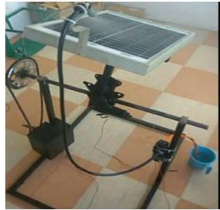
Fig.5: Use of washer for dust cleaning
