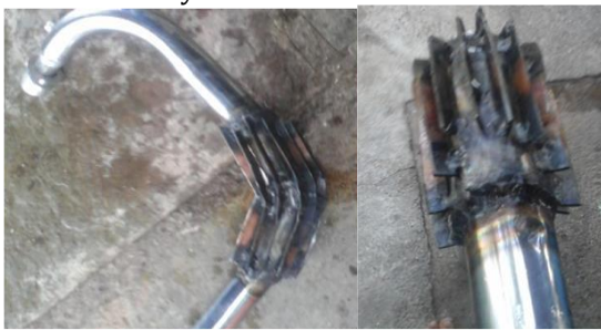
Fig.2 Fins on silencer
