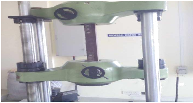
Fig. 3.1 Specimen grip assembly UTM Table in 3.1 Experimental Results
