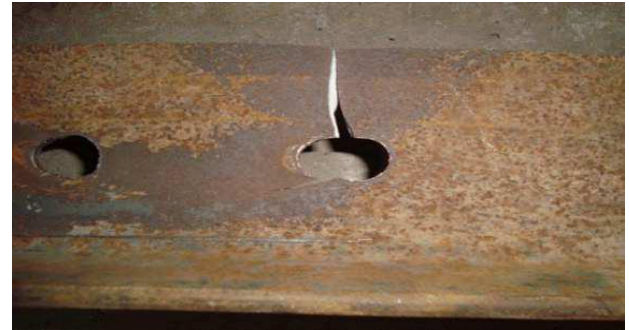
Fig. 4.1 Partial net section ruptures, with small eccentricity
