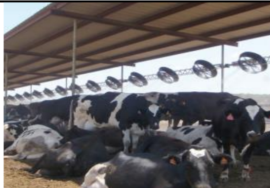
Fig 3. Flip Fan system cooling cows under a dry-lot shade
