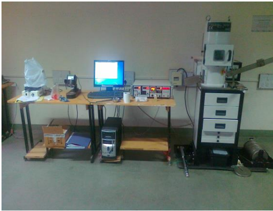
Fig.1 Four ball test rig set up
