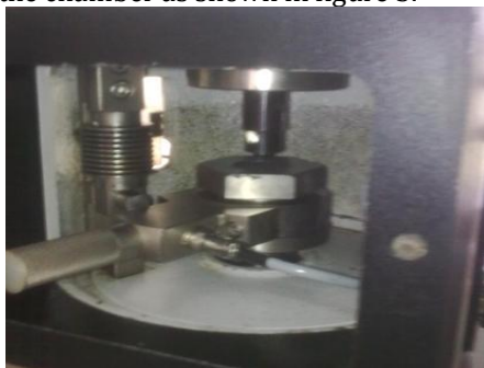
Fig. 3 Installation of oil cup assembly
