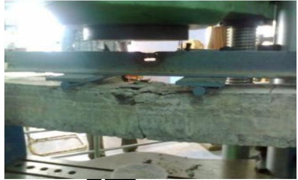
Fig. Cracks Occurred In Beam Specimen
