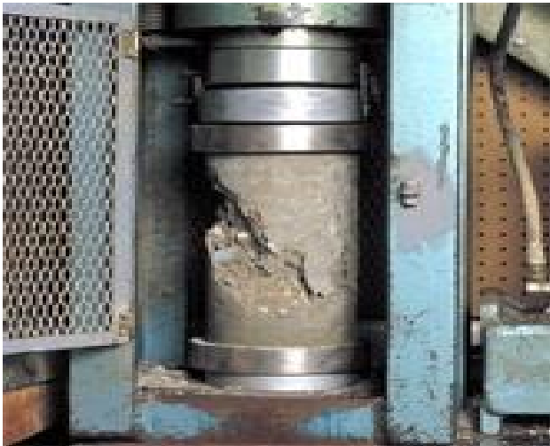
Fig. Crack occurred inside the cylinder
