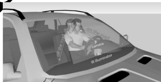
Figure 1: Eyes off the road (EOR) detection system.
