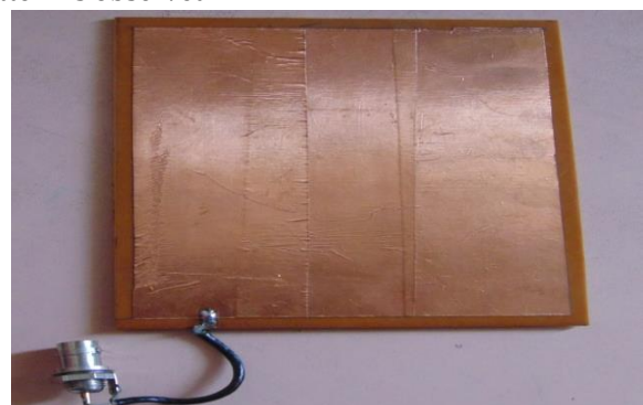
Figure.4. Fabricated patch antenna.
