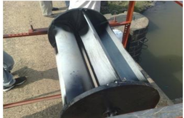
Fig. 22 Water wheel Fabricated by authors
