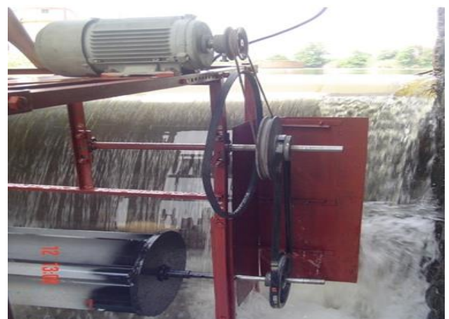
Fig. 23 Complete setup of the Pico Hydro unit
