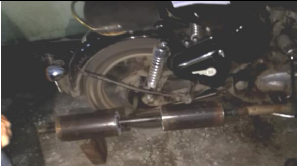
Plate 3. Measurement of sound level by using Double expansion chamber.
