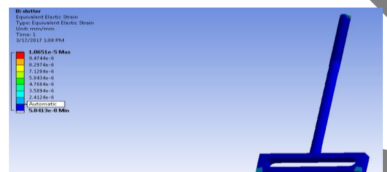
Figure 6.2: Static Structural analysis of slotter with connecting rod.
