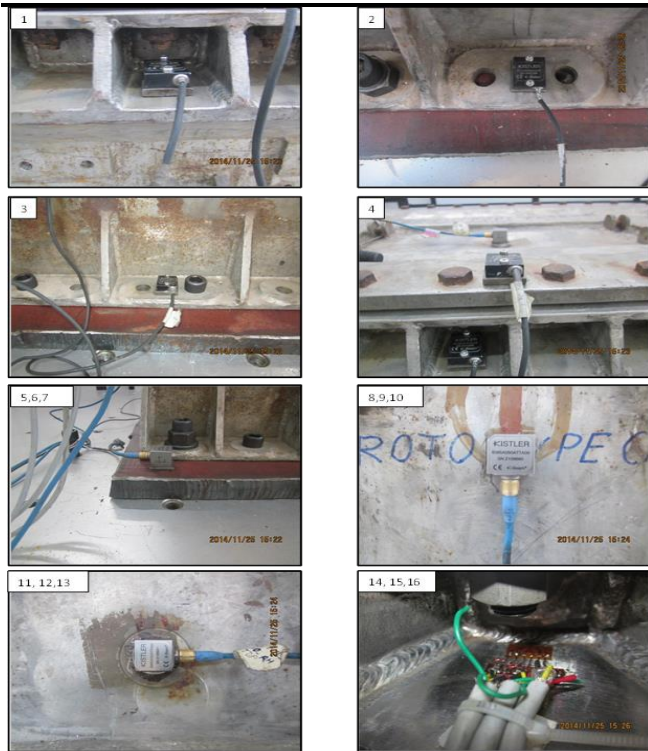
Fig. 4. Transducer Locations on Container
