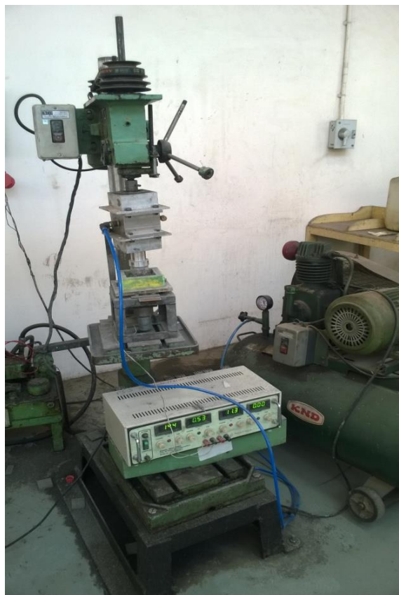
Figure 3. Experimental setup for vibration assisted gasbag polishing process
