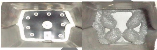
Fig. 23 Images of metal & plastic baffles after heat cycle fixed at the same place in same section
