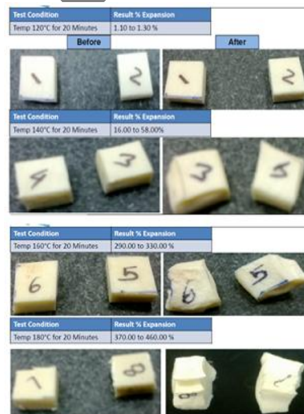
Fig. 9 Expansion behavior of material
