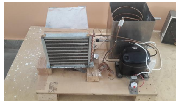
Fig 2 Experimental Set up of Evaporative Water Generation.
