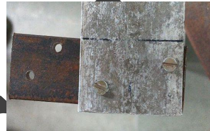
Figure 8 - Provision for attaching the absorber beam
