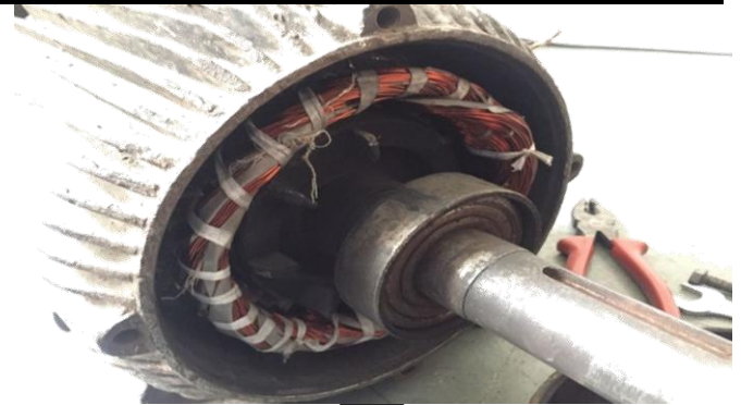
Fig No. 3: The implemented redesigned Induction motor – welding transformer model
