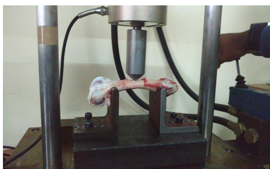
Fig. 4 shows the testing is carried in position PA (posteroanterior)
