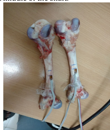
Fig. 6 Strain gauge mounted on femur bone
