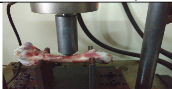
Fig. 5 shows the testing is carried in position AP (anteroposterior)
