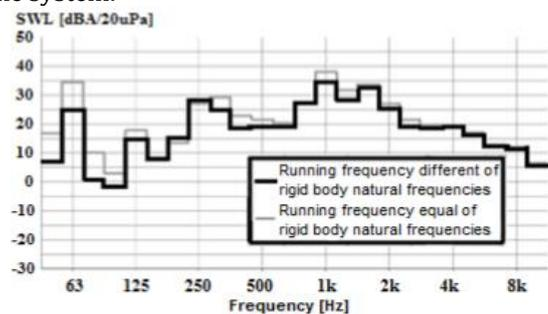
Fig. 2. Low frequency noise optimization with a good choice of grommets.
