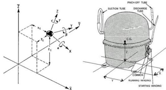
Fig. 4. Coordinate system notation of isolator location
