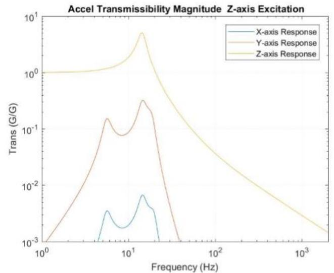
Fig. 10. Transmissibility vs Frequency graph of neoprene rubber
