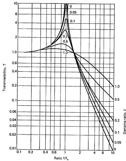
Fig. 17. Transmissibility vs. Frequency ratio graph
