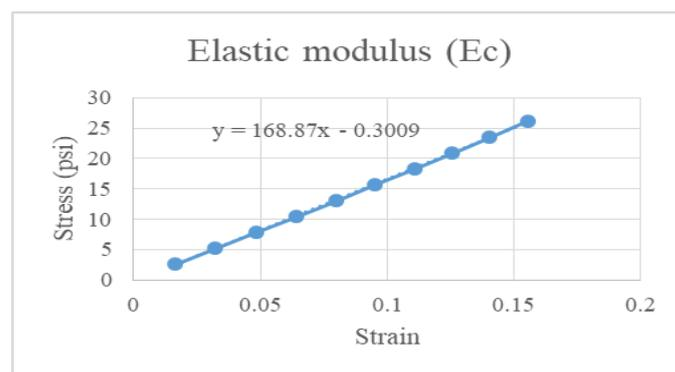
Fig. 13. Stress-strain graph of neoprene rubber
