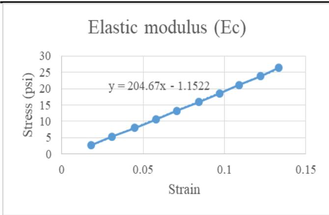
Fig. 15. Stress-strain graph of EPDM rubber
