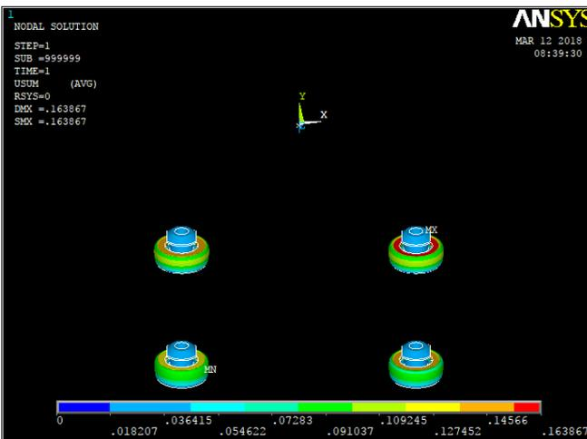
Fig. 7. Static displacement analysis of neoprene isolators
