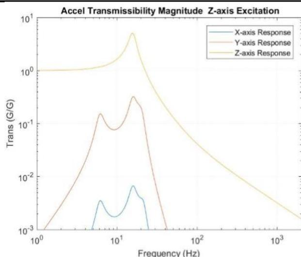
Fig. 12. Transmissibility vs Frequency graph of natural rubber
