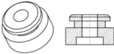
Fig. 16. Isolator geometries
