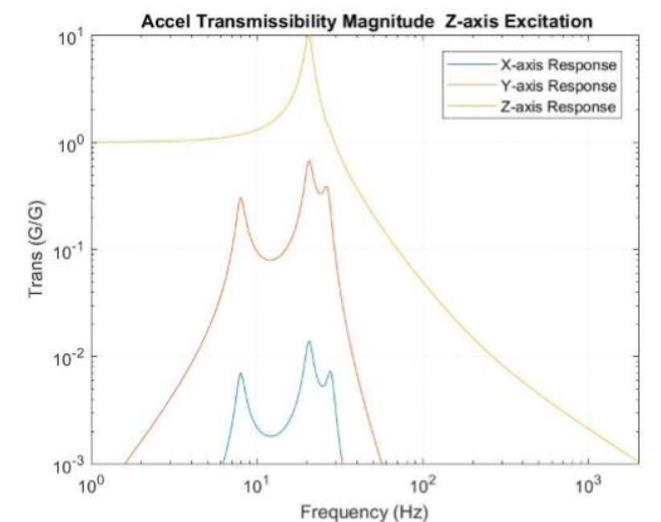
Fig. 11. Transmissibility vs Frequency graph of natural rubber
