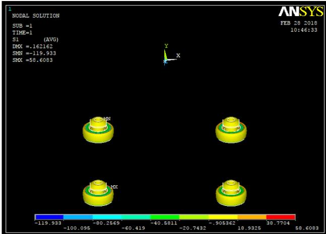
Fig. 6. Static stress analysis of neoprene isolators
