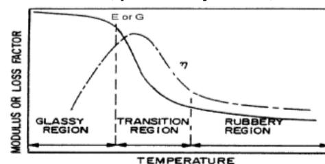
Fig. 3. The Young Modulus and the Loss Factor vs. the temperature.
