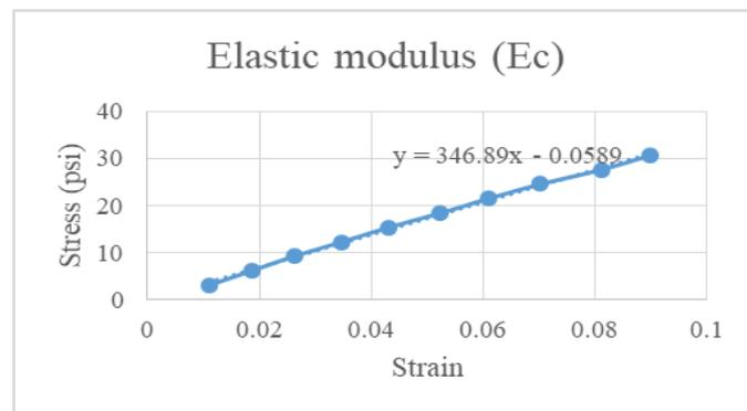
Fig. 14. Stress-strain graph of natural rubber
