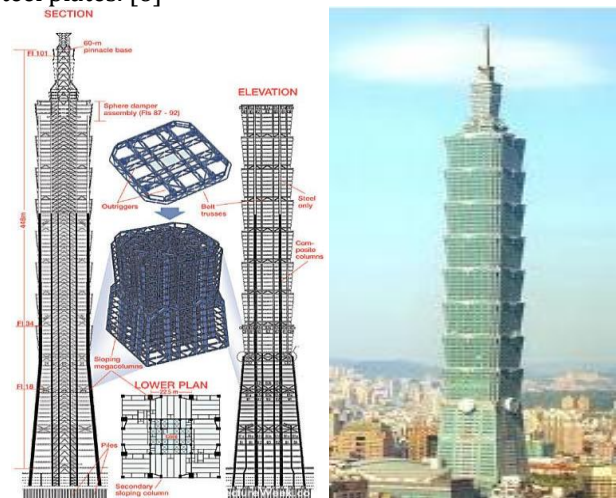
Fig.3. Structural System at Taipei Tower Source: http://delhitasa.blogspot.in/2011/12/taipei-101-taiwan-building.html https://en.wikiarquitectura.com/building/taipei-101/
