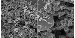
Fig. 1: SEM images of 80-nm Al particles mixed with MoO3 particles.[19].
