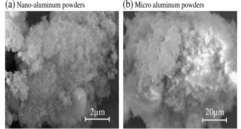
Fig. 2: Nano-aluminium powders and Micro aluminium powders [4]
