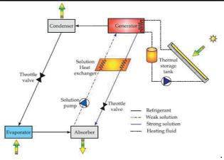
Fig. 2: Schematic Diagram Of Solar Absorption Refrigeration System[2] V.SOLAR VAPOUR ABSORPTION REFRIGERATION
