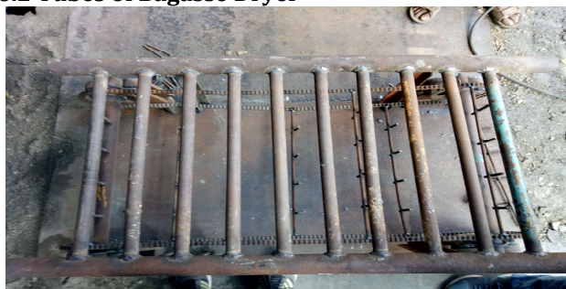
Figure 3.6.2: Tubes of Bagasse Dryer
