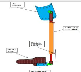
Figure 2: Schematic Diagram of Hydraulic Mechanism
