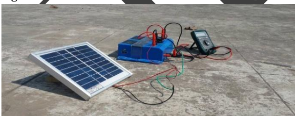
Fig. 5 PV collector performance evaluation without use of concentrators
