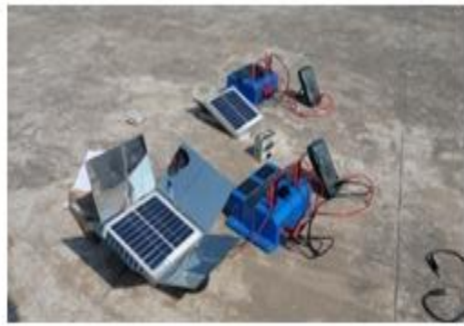
Fig. 2. Mirror augmented solar panel with regular solar panel
