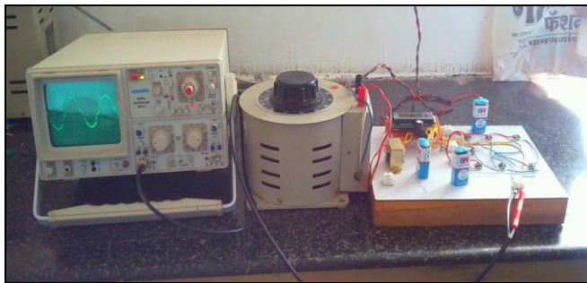
Fig. 10 Complete assembly of the experimental setup of 7-level inverter with output waveform.
