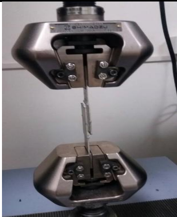
Fig.4: The photograph of specimen loaded on the 10 ton load cell UTM.
