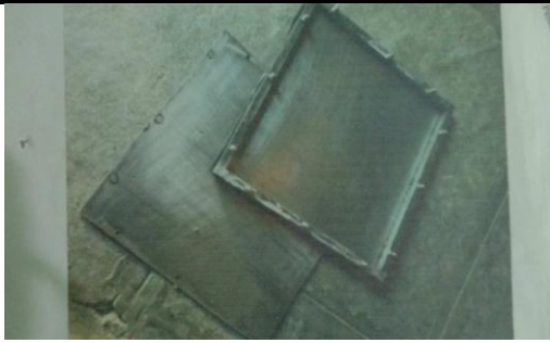
Figure 1 Mould for casting of plastic tiles
