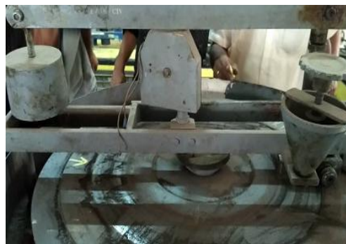
Fig. 6 : Abrasion test carried out on plastic tiles at DYPCOE, Akurdi TOM laboratory.
