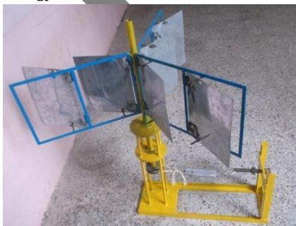
Figure 3: Photograph of Porthole Type Vertical Axis Wind Turbine (PTVAWT)
