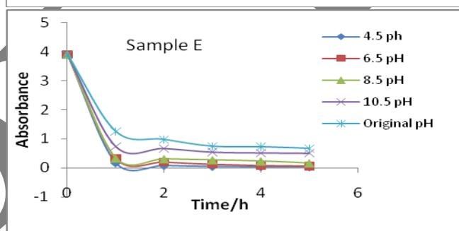
Fig.7 Graph showing the effect of pH on degradation of R6G for pure and doped cadmium sulphide.
