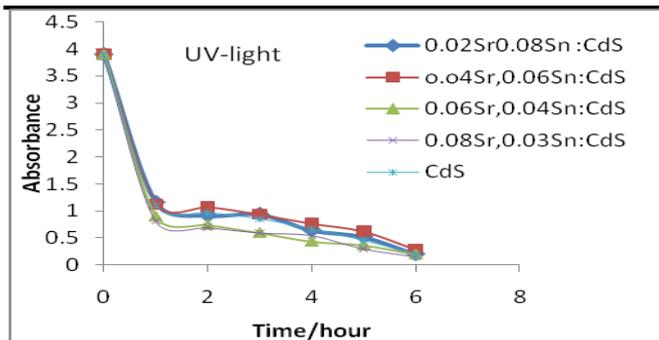
Fig. 6 b. Photocatalytic activity of Sr and Sn doped and pure CdS in UV light
