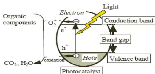
Fig. 2. Mechanism of Photocatalytic activity of photocatalyst
