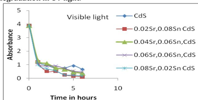
Fig. 6 a. Photocatalytic activity of Sr and Sn doped and pure CdS in Visible light
