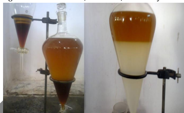
Figure 1.3: Separation of glycerol and Rice Bran oil Methyl Ester (ROME).
